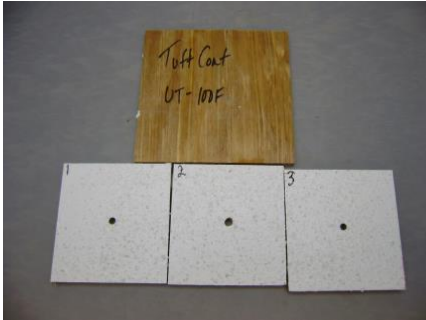
Photo No. 1 Tuff Coat UT-100 Samples, Pre-Test ASTM D 4060
